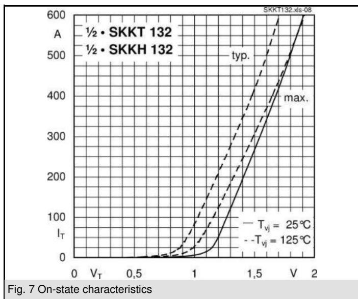
Fig. 7 On-state characteristics
