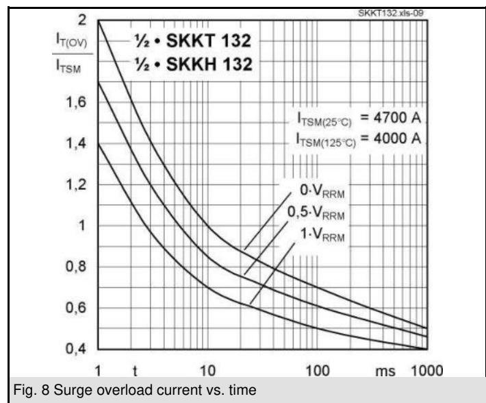
Fig. 8 Surge overload current vs. time
